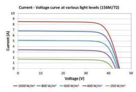
Ave. efficiency reduction of <5% at 200W/m<sup>2</sup> according to IEC 60904-1:2006
